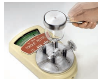
Stem twisting test
